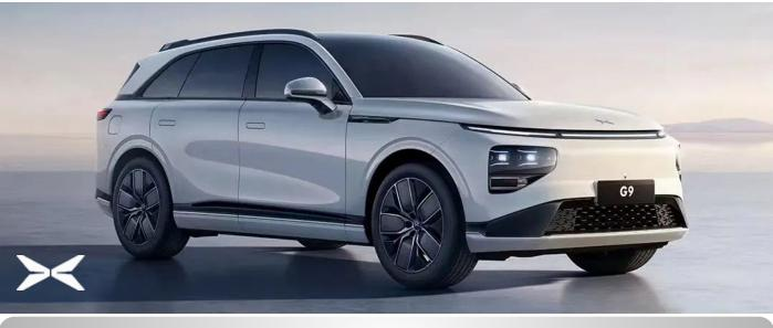
Xpeng G9- Powered by 100 kWh Battery pack Range- 600-650 km, Supercharge -800V/480kW (200 km in 5 min)
